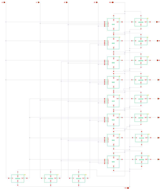
Fig 3: Decoder Implementation
